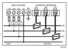
Fig. 6. 3-Phase, 4-Wire Installation Diagram
