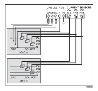
Fig. 9. Multiple Loads with one Meter
