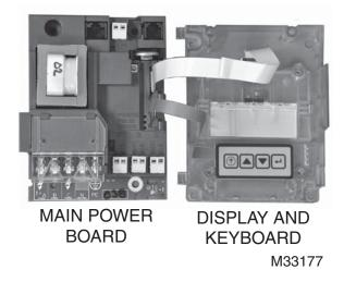
Fig. 1. Power Supply Board and Display Board
