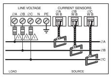
Fig. 7. 3-Phase, 3-Wire Installation Diagram
